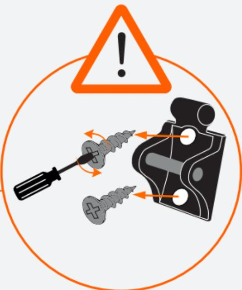
**ENG:** Replace the screws with the ones supplied for every forward lean adjustment. We recommend to apply Arexons System 52A70 thread lock. Screw them in with 4 N m of torque using a PH2 tip.
